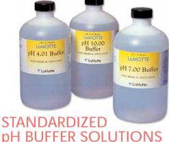
For use in calibration of pH meters. Ordering information for all buffers is listed.
